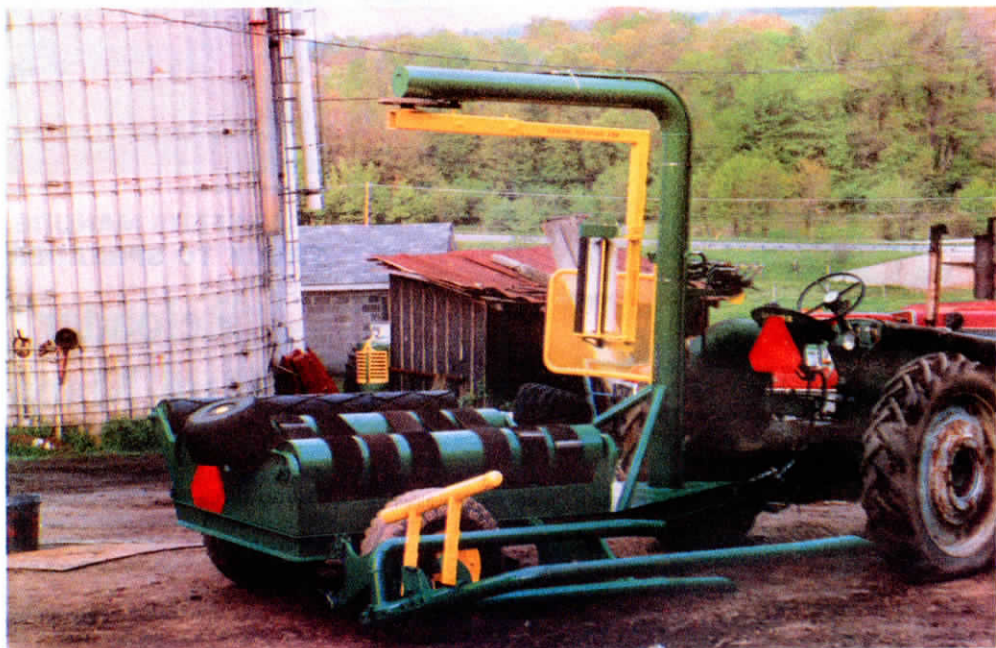
Steyer's machine has stationary turntable and plastic-wrap arm that rotates around bale. Hydraulic fork sets bale on turntable.
