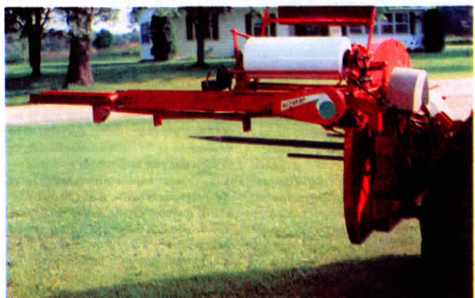
When operator raises bale after spearing it, bale starts rotating and is automatically wrapped.
