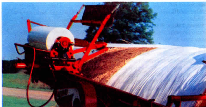
Photo shows "smoother" that presses end of plastic against bale after it's cut.
